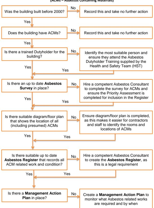
Asbestos Management Flow Chart (ACMs – Asbestos Containing Materials)
